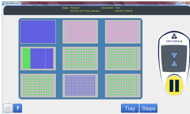
Figure 3 Screenshot from TRILUTION® micro running a Normalization Assistant protocol. The PIPETMAX® tray holds up to nine bed elements, providing flexibility in experimental design.
